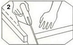
**2** Remove the door from its hinges and saw along a line parallel to the mark and 5mm above it to allow 5mm clearance between the door bottom and the rear upstand of the door sill. Smooth down the sawn surface with sandpaper. For ideal operation gloss paint or varnish the surface to ensure surface is smooth.
