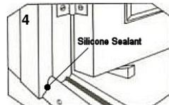
**4** Rehang the door and place door sill in position. Ensure that the door opens and closes freely and that the front face of the door butts up to the front inside edge of the door sill all along its length. Mark through fixing holes for pre-drilling the threshold. If the threshold is not of wood these holes will have to be plugged to accept the screw.
