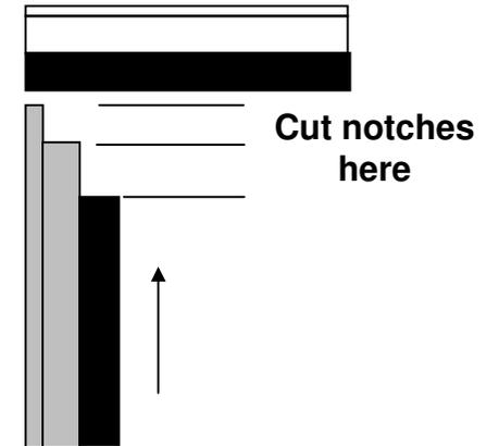
When the top piece of the XP ADS excluder has been fitted to the top of the door frame, the side pieces can then be notch cut to create a neat, efficient seal.
